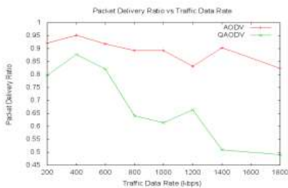
Fig. 12. Packet Delivery Ratio versus CBR
